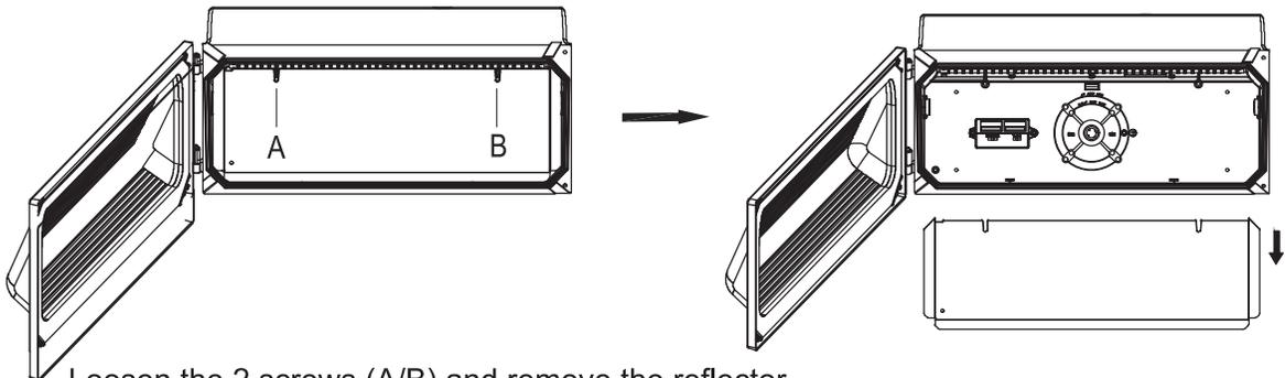
Loosen the 2 screws (A/B) and remove the reflector.
