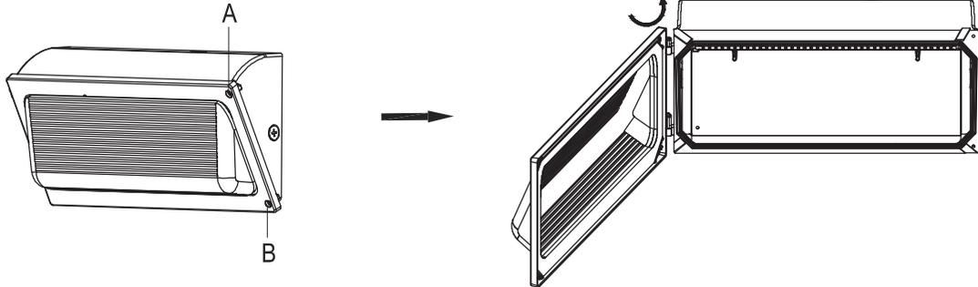
Loosen the 2x M5 crews (A/B) and open the fixture.
