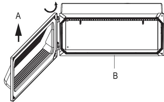
Put part A back onto the hinge of part B.
