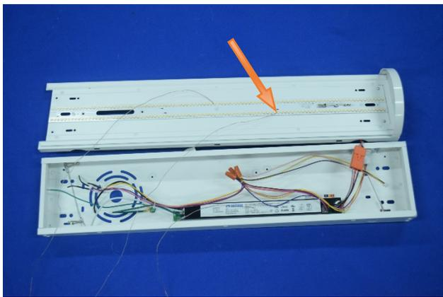
Driver Case Measurement Point T<sub>c</sub>
