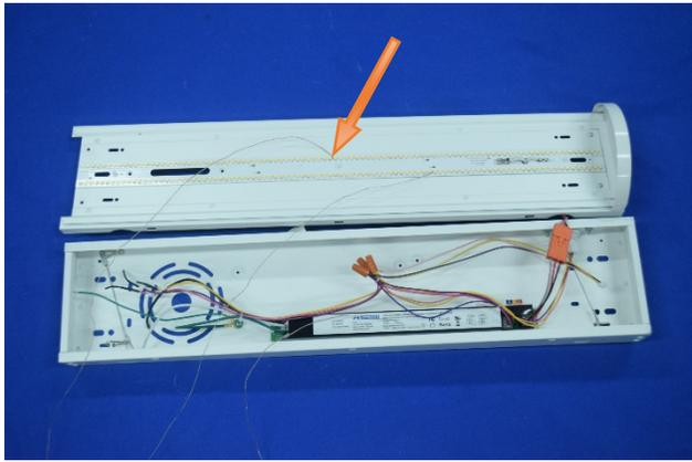
Temperature measurement point on TMP<sub>LED#2</sub>
