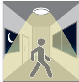
With insufficient daylight (<20 lux), when motion detected, light turns ON.
