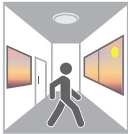
With sufficient daylight (>20 lux), even when motion detected, light remains OFF.
