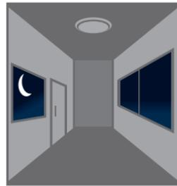
After the last detection and the present hold time (3 mins), has elapsed, light turns OFF.
