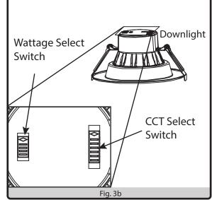
4. Carefully place all wires safely up into the junction box and replace the cover panel. Fold up both spring brackets, located on the sides of the downlight, and insert the downlight up through the ceiling while letting the Spring brackets close and latch onto the upper surface of the ceiling panel. Make sure the fixture is properly secured to the ceiling before releasing support and completing install.
